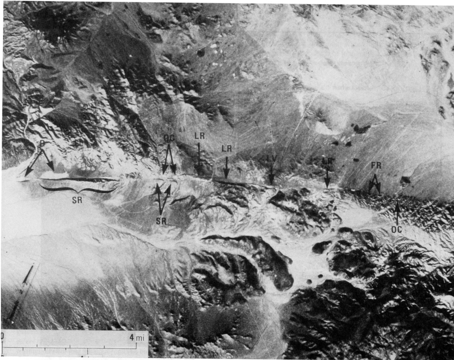
Figure 13-3 Satellite photograph of the topographic features along the left-lateral, strike-slip Garlock fault, in the Mojave Desert of southern California. The following features indicate that the fault is active: D = depression, SR = shutter ridge, OC = offset channel, LR = linear ridge, LV = linear valley, FR = faceted ridge. From Merifield and Lamar (1975, Figure 2). Courtesy P. M. Merifield, UCLA.
