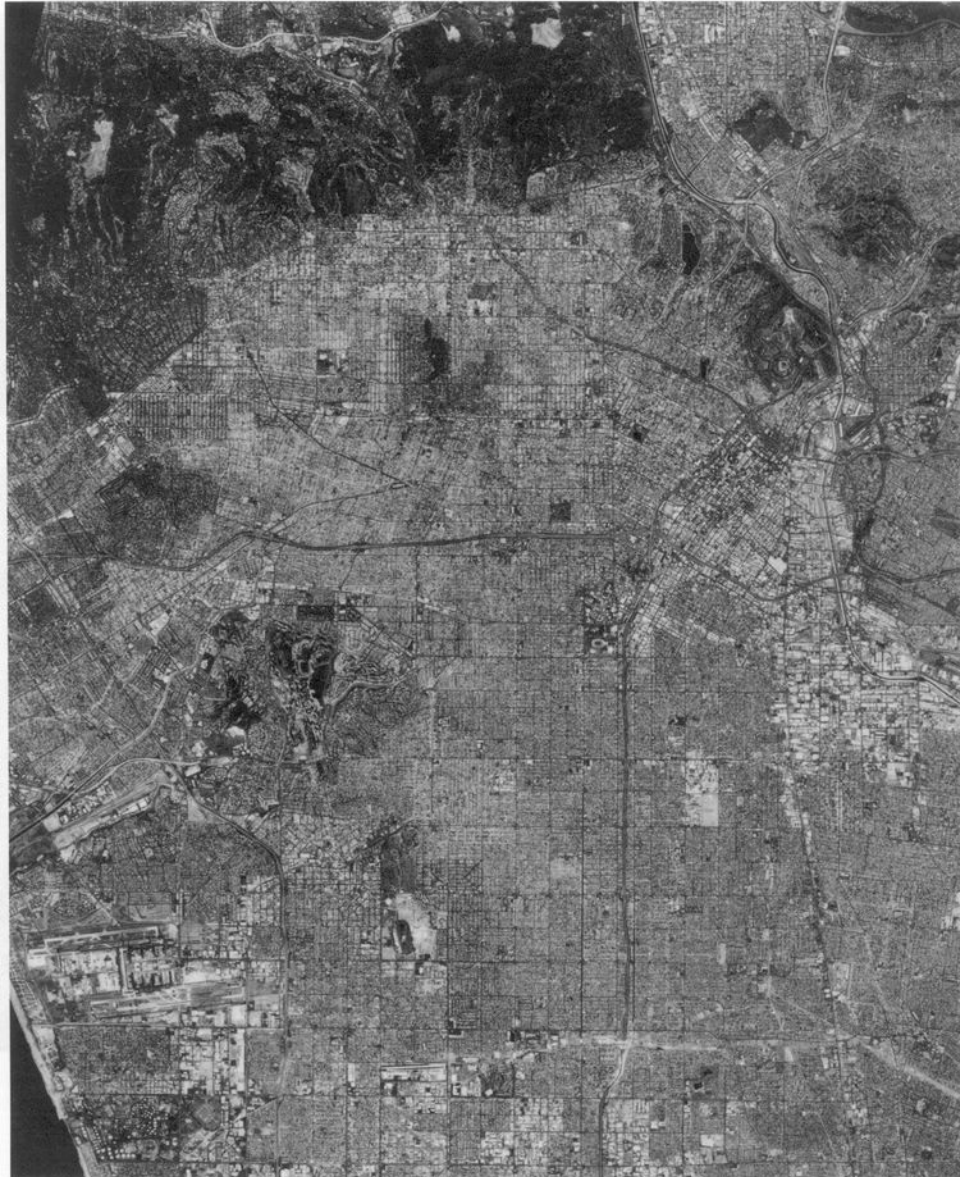
Figure 12-3 SPOT pan image (10-m resolution) of the western portion of the Los Angeles region, used for the level II land-use classification. Image was acquired July 20, 1986.
