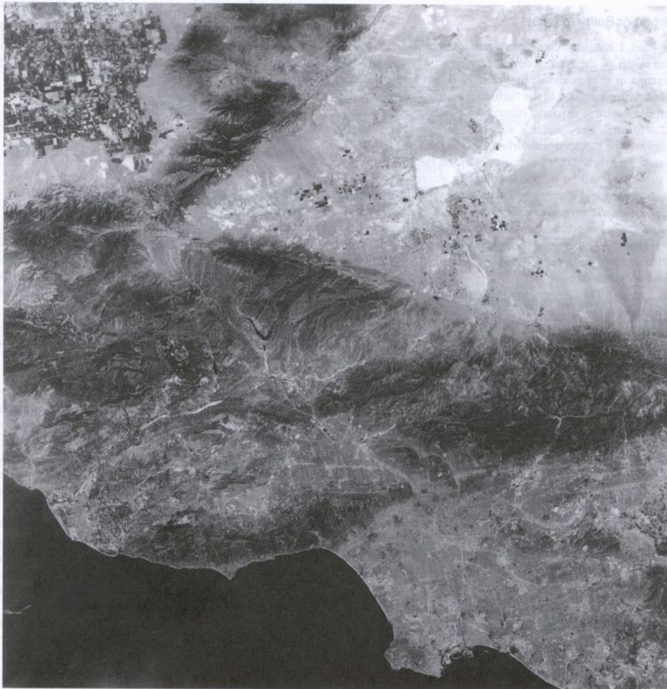
Figure 12-1 Landsat TM band 3 (red) image of the Los Angeles region, used for level I land-use classification. Image was acquired July 3, 1985.
