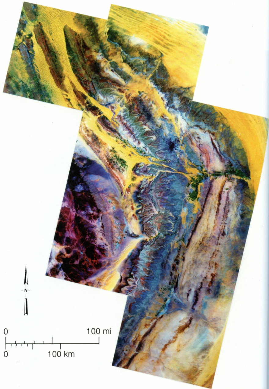
Plate 4 Analog mosaic of the Central Arabian Arch compiled from Landsat TM 2-4-7 prints.
