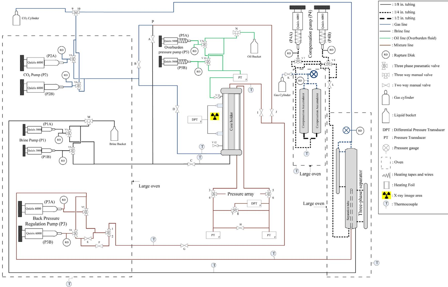
Fig. 2. Schematic flow diagram of the experimental setup used in this work (Piri, 2012).
