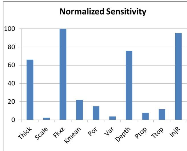
Fig. 5. The computed sensitivity index of the output variable (percent CO<sub>2</sub> leakage) to uncertain input parameter varied in the global sensitivity analysis.
