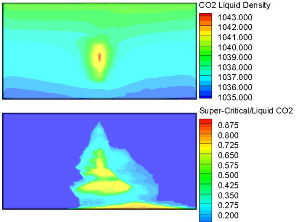
Fig. 7. The simulated CO<sub>2</sub> liquid density (upper) and CO<sub>2</sub> saturation (lower) in a vertical cross section (from MC run 22).
