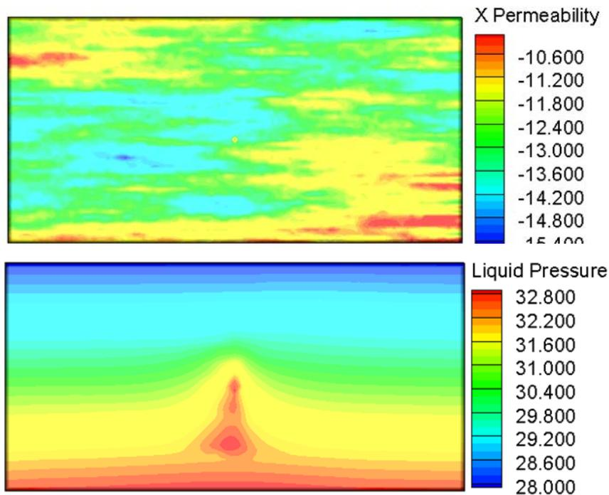
Fig. 6. Horizontal permeability ( $\log_{10}$ ) field (upper) and the simulated CO<sub>2</sub> liquid pressure (MPa) (lower), in a vertical cross section (from MC run 22).
