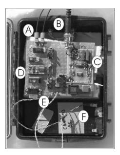
In the figure: A labels the fiber optic links for triggering the transmitters, B is the receiving antenna connection, C is the 100MHz amplifier and A to D converter, D is the microcontroller, real time clock and memory section, E is the serial communication section and F is the gell-cell battery. The unit is contained in a water-proof enclosure.
