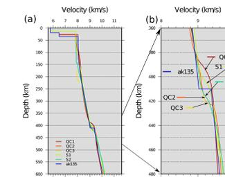
Figure 10. Tau-p migrated velocity results for five earthquakes. (a) Velocity to 600 km depth. (b) Close-up of 410-km discontinuity velocity profiles.
