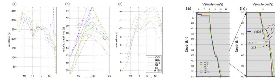
Figure 9. Summary of observations for five earthquakes. (a) Ray parameter vs P-wave travel time. (b) Epicentral distance vs travel time reduced by 11.2 s/deg. (c) Ray parameter ( $p$ ) vs time-intercept ( $\tau$ ) reduced by  $\tau = -17.2 p + 245$  (s).
