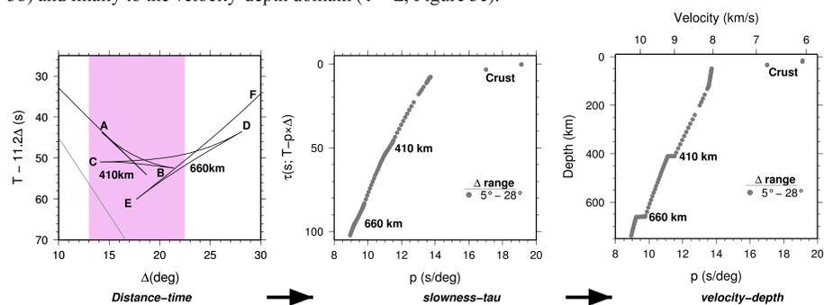
Figure 3: (a) Reduced-travel-time curves for a distance range of  $10^\circ - 30^\circ$  (IASPEI91 reference model). The region of 410 km triplications are highlighted. (b) The corresponding  $D - \tau$  curve, where  $\tau$  is the intercept-time. (c) The velocity-depth profile that results from migrating the  $p - \tau$  curve.
